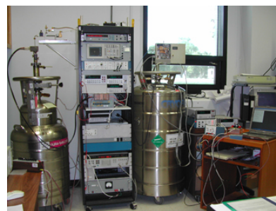
JJ voltage standard \Delta V/V < 10^{-10}
